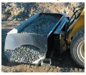
The Side Dump Bucket is designed with a quick attach that allows it to mount to most skidsteers. The hydraulic lines plug directly into your remotes just like any other skid steer attachment. The Side Dump Bucket is made with a heavy duty tubular steel frame, continuous welds and gusseted for strength. The cutting edge bolts on for ease of maintenance and replacement.
