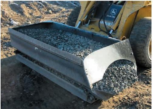
The side dump feature allows the skid steer operator to see where the material is being placed resulting in neater, more controlled placement of the material. It also enables the operator to load the material into the Side Dump Bucket and then load the paving/curbing machine while moving only in a straight line. This reduces spillage of material and eliminates the need for cleanup along the work route.
