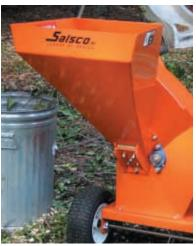
The infeed hopper opening is wide and will accept bushy branches, gravity feed makes it easy to run material through the chipping disc.
