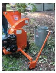
Exhaust chute easily fits over the standard trash can or even a 30-gallon container for easy debris removal.
