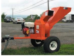
Available as an option, the *Transport Wheel Kit* makes the unit easy to tow on the road. 2" Ball Coupler and Tow Chains are also provided with the
