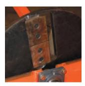
6 - 1/2" Thick, double-sided, chip blades, segmented into 3-knife pockets. Easy access to blades through 1/4" thick steel impeller housing.
