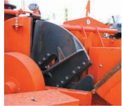
1/2" Thick, Double Sided Chip Blades! 2" Thick x 32" Diameter Impeller1
