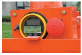
Above - The feed sensing option counts the impeller R.P.M. and recognizes when the tractor is getting loaded up, due to a combination of large, long logs and not enough horsepower. If this happens the Feed Sensing will stop the feed roll and allow the tractor to catch up.
