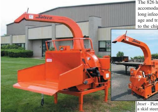
The 826 has an extra wide infeed hopper to accommodate brushy material, and an extra long infeed tray that folds up for ease of storage and transportation. The infeed opening to the chipper disc is 6" high by 12" wide.
