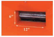
Above - The infeed opening on the 826 is 6" high x 12" wide. This extra wide opening accommodates brushy material and reduces the pruning and trimming.
