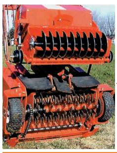
Cutter blades are spring loaded to provide maximum cutting pressure while allowing blades to give, should they hit a hard object. Mud Scrapers keep seed discs clean while seed tubes deliver seed to discs for planting. Tires are pneumatic, turfsavers and tire guards protect tires. Protective rubber debris guards provide extra protection for the operator. Standard cutter blades are 11 gauge hardened steel.
