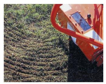
The 355/2000 plants rows on 2" centers and plants a 20" seed bed. *Slicer depth is infinitely adjustable up to 2-1/2*".
