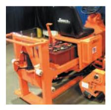
When batteries need to be recharged, the Battery Tray Cart easily rolls into place under the tray. Un-latch the tray and lock it into place on the cart, to transport the discharged battery pack to the Battery Tray Holder. Plug in the charger to the Battery Tray and use the Battery Tray Cart to transport the charged Battery Pack to replace the removed Battery Pack in the QC.
