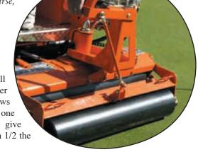
The optional Spike-Air Kit when used on the green will gently spike the green to allow water & oxygen penetration through the crust to the roots of the plant.
