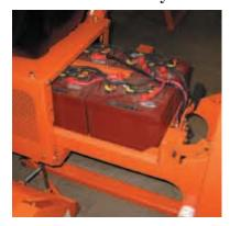
The Battery Tray, complete with Batteries and Watering system, locks in place in the battery compartment under the seat of the QC.
