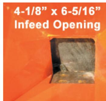
Chipper **infeed opening at the impeller is 4-1/8" x 6-5/16"**, and will easily accommodate up to **4" diameter round wood**. Bed knife is adjustable & sharpenable.
