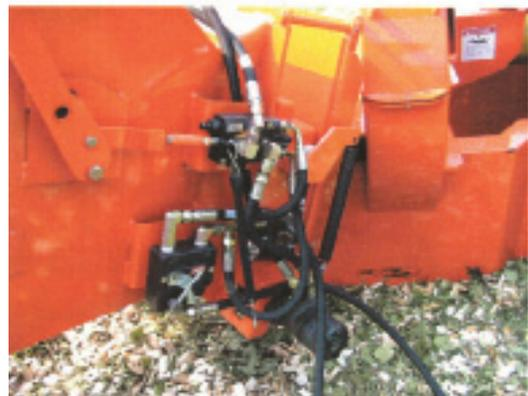
Flow Control Valve (Standard Equipment) provides infinite speed control to accommodate all tractors.
