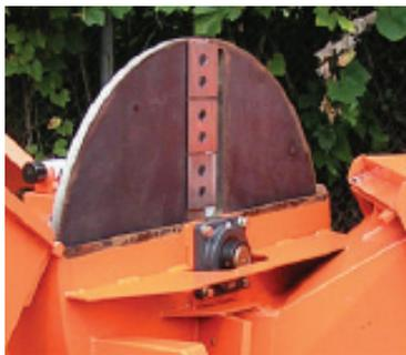
4 Bolt, cast iron, self aligning, greaseable bearings! Replaceable, sharpenable, adjustable steel bed knife!
