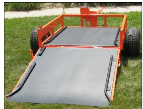
Transport Trailer is standard and has many other uses around the golf course. Salsco trailers have roller assist rails to help guide the operator on and off the trailer.
