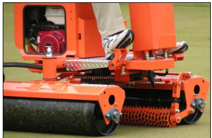
Both rolls are driven for positive traction, and both rolls oscillate. Rolls are in full contact with the ground 100% of the time.
