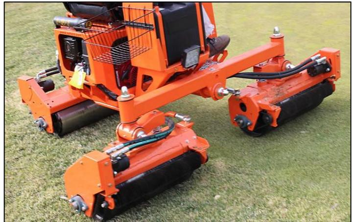
Three (3) oscillating and articulating steel rolls, driven for positive traction. All rolls are in full contact with the around 100% of the time.
