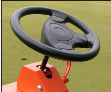
Articulated Steering / Automotive Type, Tilt Steering Wheel
