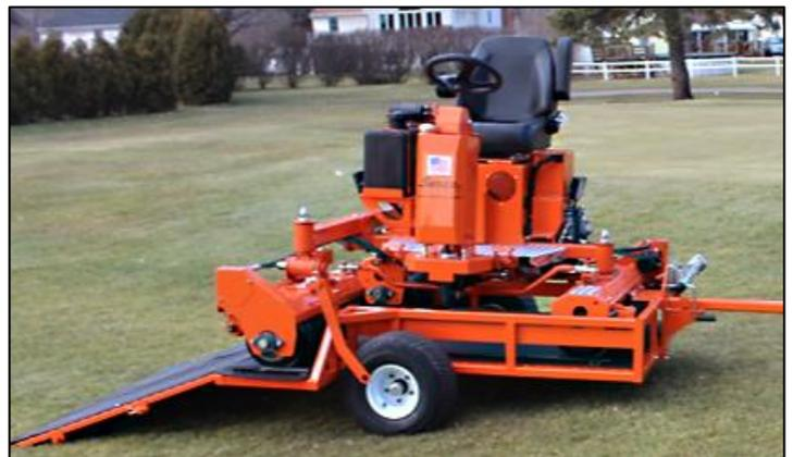
The Transport Trailer is standard and has many other uses around the golf course. Dual lock latch tailgate ramp with a full 1/4" thick traction mat on both the trailer box and tailgate, with loading guide rails.
