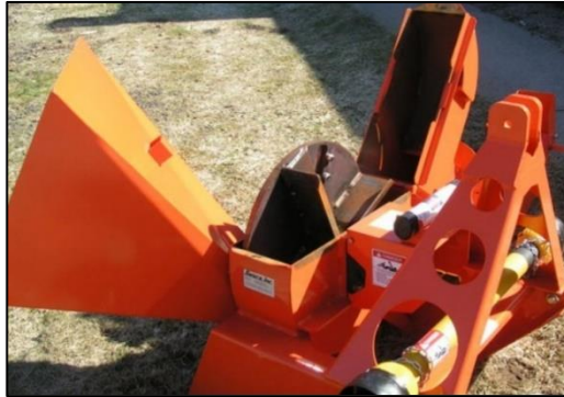
Impeller Housing unbolts to allow easy access to the Impeller
