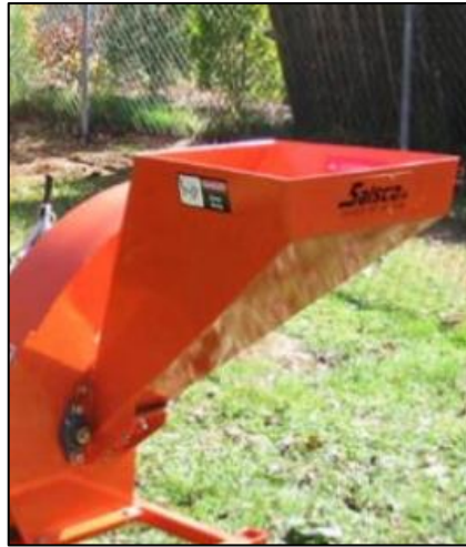
Extra-large Infeed Hopper accommodates bushy branches
