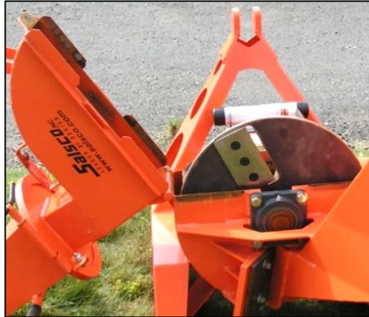
210 lb. Impeller with three (3) welded and gusseted exhaust paddles. Impeller Housing easily opens to allow access to the Impeller for maintenance
