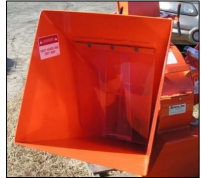
Extra wide Infeed Chute with curtains helps protect operator from fly-back of material
