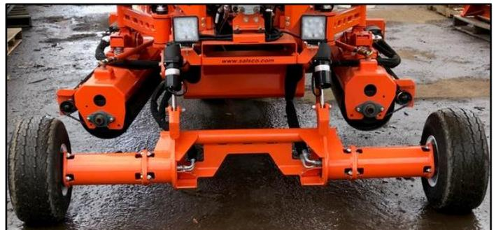
**Rear Wheel Extension** adds stability when using on hilly terrain.
