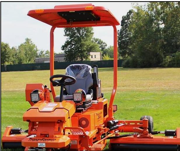
**Cool Top w/Fan** is a factory-installed option that allows extra relief from the sun.
