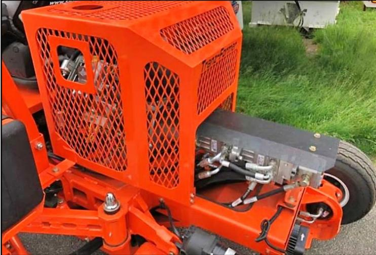
**Engine and Engine Cover:** We moved the engine and pumps to the back of the machine for easier and faster access for maintenance. We also removed many hoses avoiding potential leaks! With the engine and pumps at the rear of the machine, heat and noise dissipate.
