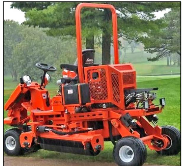
**Transport Mode.** When wheels are down, it's in the transport mode; Wheels up is the roll mode. Transport speed is 10 mph.
