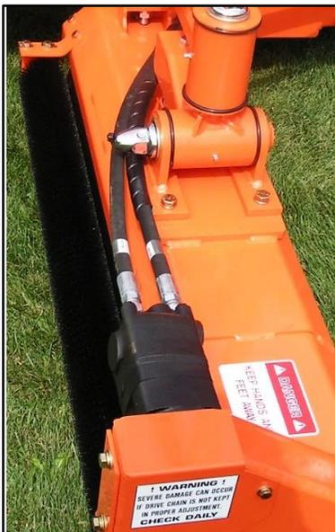
**Rotary Brush System** is a standard feature that helps prevent sand and loose grass from building up on the rolls. Brushes on all three rolls.
