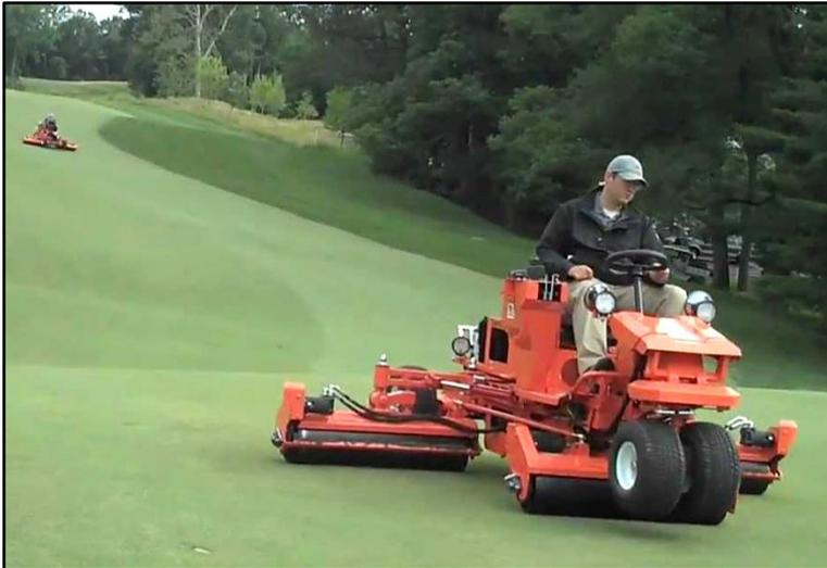
**Three (3) Steel Rolls** are driven for positive traction and extremely capable of handling hilly terrain.
