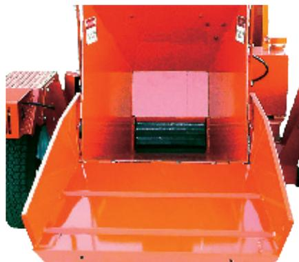
Infeed opening is **7" High x 8" Wide**. Extra wide infeed tray opens up to a full 49" from the infeed rolls.
