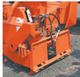
The Skid Steer Plate, complete with all necessary hydraulics is available as an option and can be used with either high or low flow.
