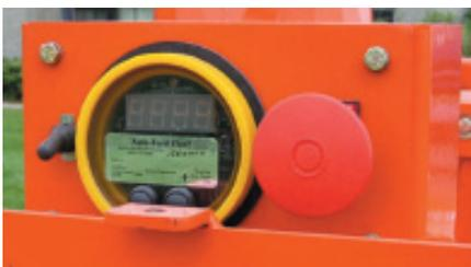
The Speed Sensing option counts the impeller RPM and when the impeller slows down, the speed sensing kicks in and stops the feed roll until it picks up the proper RPM for maximum efficient operation.
