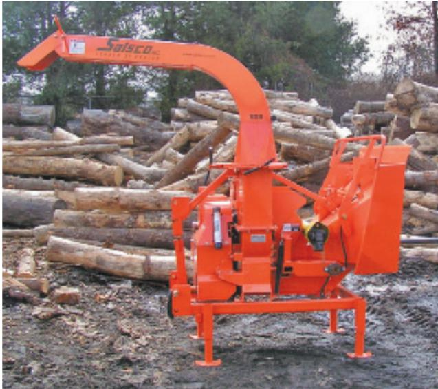
The 826PTO has a **6" high x 12" extra wide infeed opening** to accommodate brushy material, and an extra long infeed tray for safety. The infeed tray folds up for ease of storage and transportation. Minimum horsepower is 25HP at the PTO and only **requires 540 RPM**. Hydraulics are self-contained; no remote connections to the tractor are needed. The control handle is easily accessed from either side and has a slow speed, high speed, neutral and reverse.
