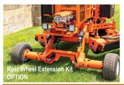
The optional Rear Wheel Extension Kit adds stability where needed, especially on steep inclines. The Rear Wheel Extension Kit can be ordered as retrofit to units in the field, or factory installed on new units.
