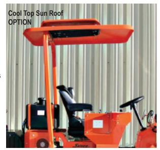
Cool Top Sun Roof option, with or without a fan, is mounted to the roll bar and can be retrofit to units in the field, as well as factory installed.
